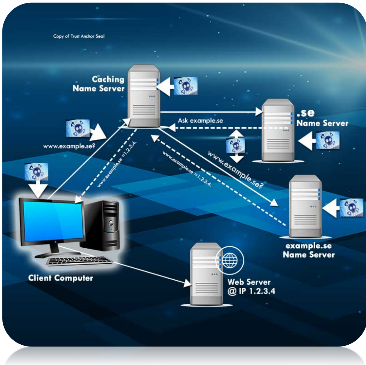
Figure 1. DNS query resolution process and potential attack targets
